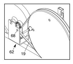
Screw. Reattach the side shields.
